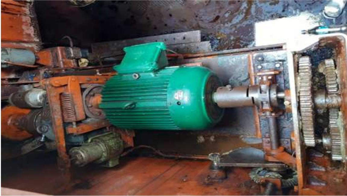
**Fig 2.18 Motor of opening arrangement of disperser valve**
