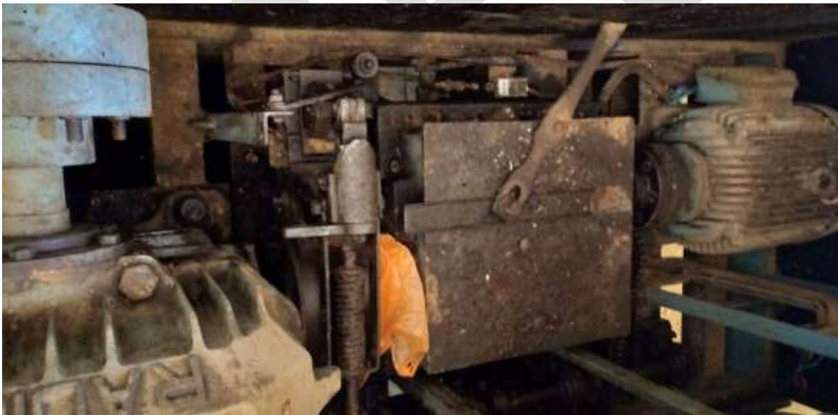
**Fig 2.20 Motor, gear and brake arrangement**
