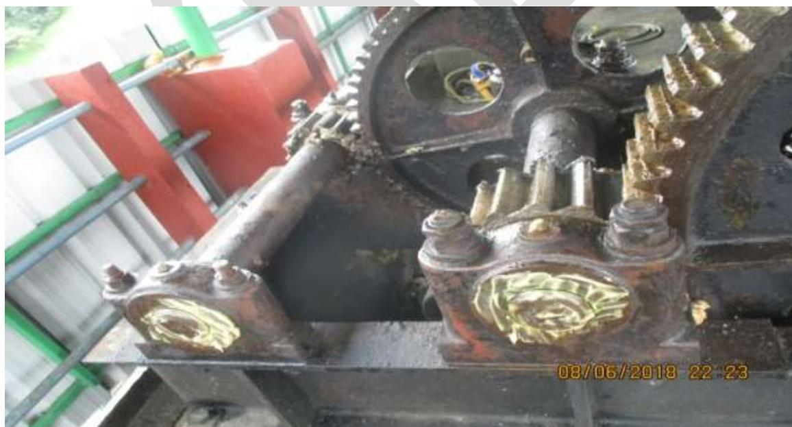
**Fig 2.7 Motor and gear box brake**
